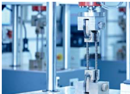
More than 25 pulser are available for testing dynamic fatigue strength according to different testing methods
